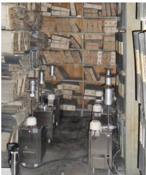
Figure 1 Sampling in the repository of the State Regional Archives in Třeboň employing Leckel LVS-3 devices.
